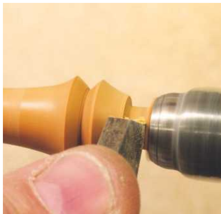
▲ Pic.26 He is turning the top spigot down to 10mm to fit into the top cross member. It can be worth taking a little tailstock pressure off at this point to prevent splitting
